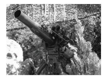
X11, an operator must peer through the weapons electronic sighting system and guide the rocket to its target. The Thermal ForwardLooking Infrared (FLIR) sighting system makes the attack roll Easy, overcomes darkness modifiers and allows the operator to see through smoke.
