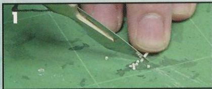
1. Using a sharp knife, begin cutting the plastic rod into slices. Try to keep the slices all the same thickness as this will make the finished piece of terrain look more realistic.
