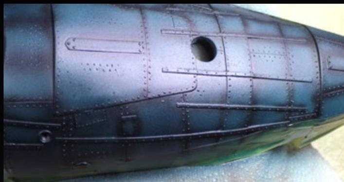
The entire hull then received a coat of translucent Prussian Blue, giving me a slightly metallic finish and then a layer of hairspray.
