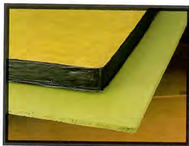
▲ Two gaming boards made from a thick sheet of polystyrene (top) and chipboard (bottom).
