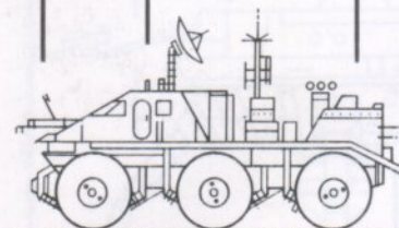
Planet Rover 2012-2020 LENGTH: 16 m WEIGHT: 8.8 tons SHIP'S COMPLEMENT: 4-6 PROPULSION: Electric
