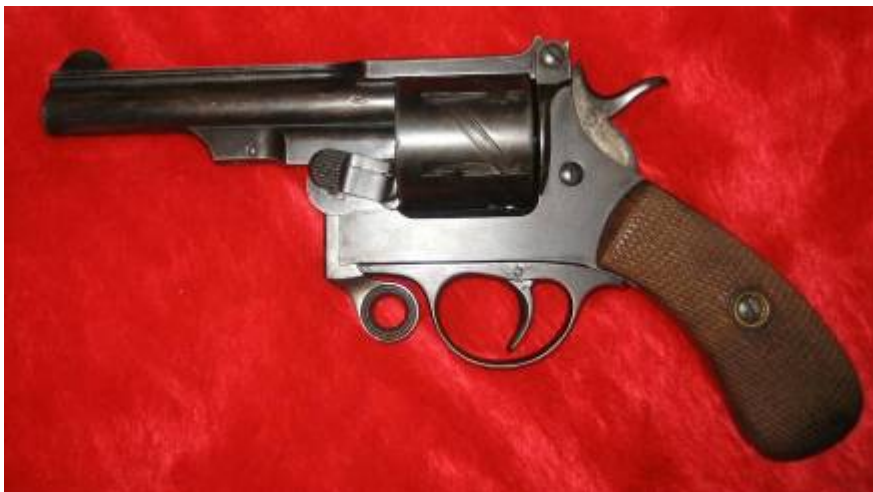
German, Mauser Zig Zag Revolver, 1878, 6 shot, 10.6 mm
