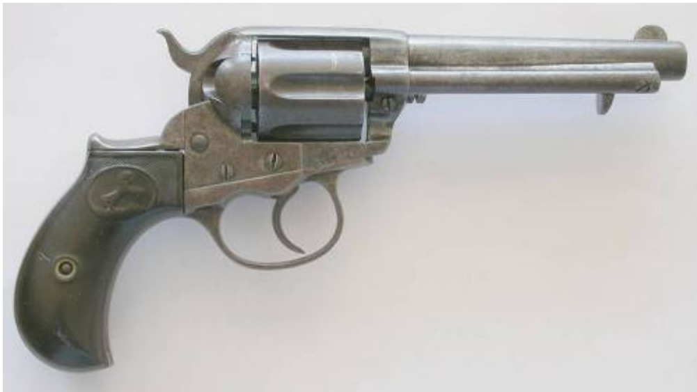
USA, Colt Thunderer Revolver, 1877-1900, double action, 6 shot, .41 caliber long and short Colt
