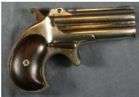
USA, Remington Double-Barrel Derringer, 1866, 2 shot, single action, .38, or .41 cal
