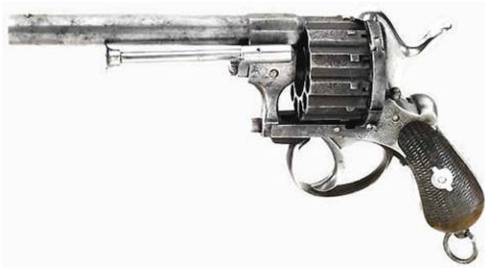
France, Lefauchaux Pin Fire Revolver, 1858, single action, 10 shot, 7mm PF
