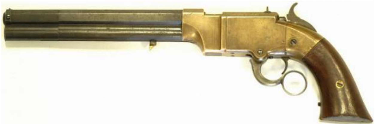
USA, Volcanic Navy Pistol, 1855, lever action, 10 shot, .41 cal Volcanic, 8" barrel, also a 8 shot, with an 6" barrel, tube mag. under the barrel
