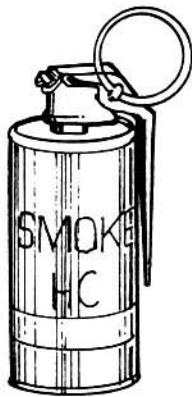
THE SAME BASIC STYLE OF CANISTER IS USED FOR SMOKE AND INCENDIARY HAND GRENADES.
