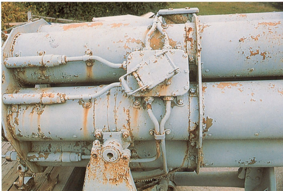
Fig.5 The launching tube assembly completed, painted and weathered. The grenades were usually painted light gray or light green, depending on the factory responsible for their production.
