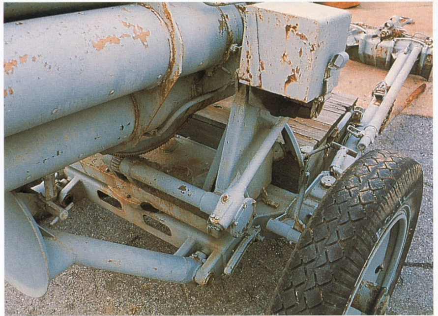
Fig.8 & 9 The carriage subassembly after finishing, ready to take the launching tubes. Intended to be shown in a stand-by launching position, the support at the front was secured in the down position, the stowed position is shown at right.
