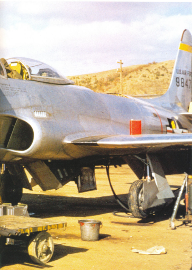
F-80 pilots rarely returned from a mission with 0.5-in ammunition to spare, for they would diligently strafe any target they could find. With its nose supported by jacks, this 8th FBS Shooting Star is having its guns replaced at the unit's Taegu base. Note that the aircraft lacks the yellow trim synonymous with 8th FBS F-80s, indicating that it was a replacement fighter recently delivered to the unit (Budd Butcher)
