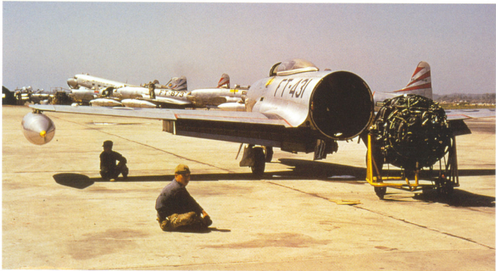
ABOVE Most of the major maintenance work carried out on the 8th FBG's F-80s was done at Iwakaze AB, although this routine engine change was taking place on the 36th FBS's flightline at Suwon (K-13) in the summer of 1952 (Don Brown)
