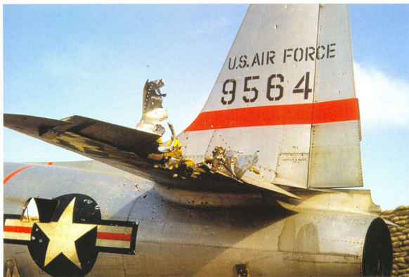
LEFT This 25th FIS jet was riddled with automatic weapons fire as it pulled out of a dive-bombing run through a valley in North Korea – the gun positions were sited on nearby ridges. If the gunner had led his target a little more, the damage would have been centred around the cockpit, and that could have been disastrous (H P Saabye)
