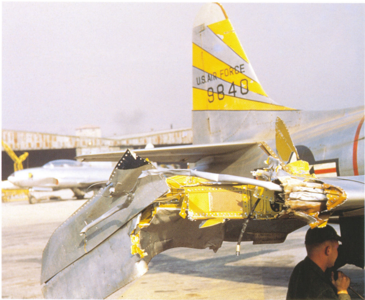
ABOVE The F-80 proved itself to be every bit as rugged as its piston-engined forebears from World War 2, being able to absorb heavy battle damage of the sort shown in this photograph. This 80th FBS fighter-bomber hit a cable while on a low-level strafing run through a mountain valley in North Korea – the pilot was still able to land the F-80 back at Suwon. The enemy's use of cables was an on-going problem for the duration of the war (Chuck Baisden)
