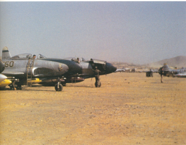
LEFT The key to the F-80's effectiveness once the Chinese entered the war was the fast turnaround, with units flying as many sorties as the maintenance people could support. These heavily-loaded 'Screamin Demons' from the 7th FBS have been rearmed with napalm and rockets for their afternoon mission against suspected troop concentrations. This deadly combination was also effective against enemy tanks that were caught out in the open (Frederic Champlin)
