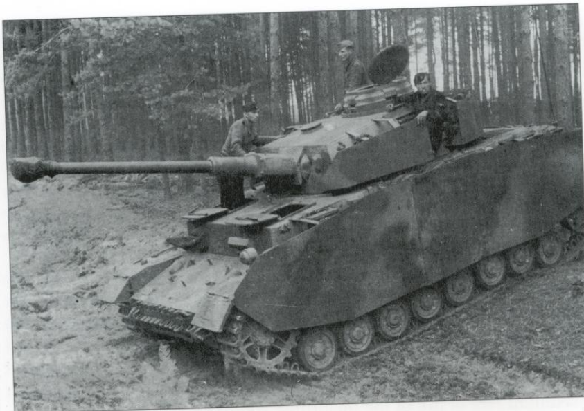
The Ausf. H had 80mm integral front armour and was fitted with side skirts and a turret girdle of spaced armour to protect it against hollow charge ammunition. The colour scheme of this particular vehicle, serving with a Waffen-SS division, is basic German dark yellow oversprayed with large dark green and rust-red patches. (Bundesarchiv)
