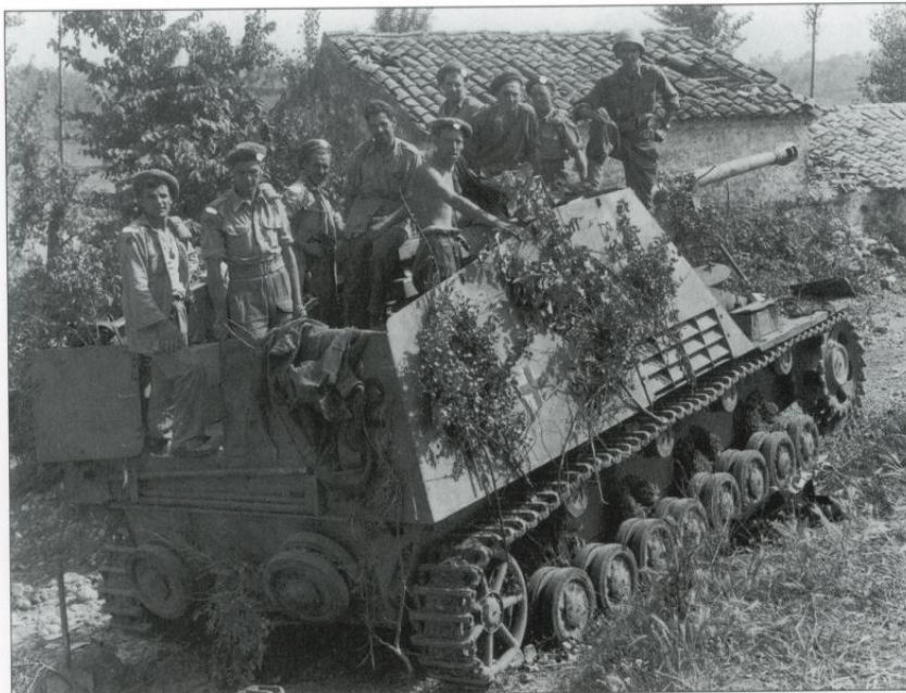
The Nashorn (Rhino) was a first-generation heavy tank destroyer and was armed with the L/71 PAK 43/1 88mm anti-tank gun. This example was stalked and killed with a PIAT by Canadian infantry near Pontecorvo, Italy. Unfortunately, the censor has erased every detail of cap badges and shoulder titles. (Public Archives of Canada)
