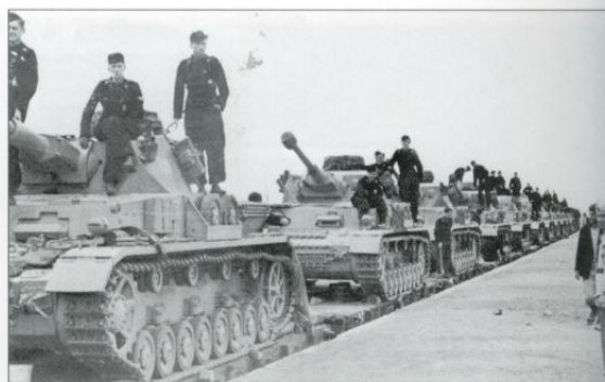
Additional 30mm appliqué frontal armour and the 75mm L/48 gun identify these Ausf. Gs in transit by rail through the Balkans. In such circumstances it was normal practice to lock the gun in elevation by means of an internal crutch. (Bundesarchiv)
