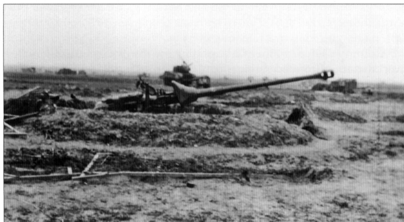
A number of these modified PaK 43/3 88mm guns were knocked out by the new Pershing tanks of the 9th Armored Division on the approaches to the Rhine. These weapons were intended for the Jagdpanser tank destroyer, but instead were adapted to a pedestal mount for use as an improvised anti-tank gun for Rhine defense. (NARA)
