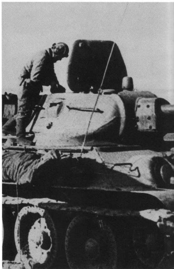
ABOVE: A T-34/76B, showing the large turret hatch that made the tank vulnerable to close range attack by infantry with grenades.
