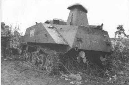
A rear view of one of the Type 2 Ka-mi amphibious tanks knocked out during the fighting at Ormoc Bay. These tanks had propellers which gave them reasonable good handling characteristics in the water during landing. The two crab-claws at the rear of the hull were used to attach the rear pontoon.
