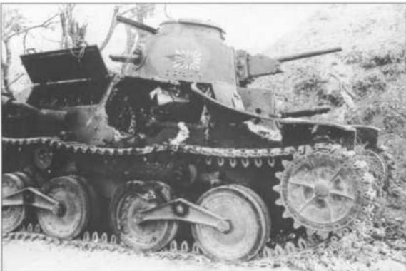
A Type 95 Ha-go light tank of the 4th Company, 9th Tank Regiment knocked out during the fighting near Black Beach 3 on Saipan on the morning of 16 June 1944. This tank appears to have been hit by an anti-tank round on the upper edge of the sponson which not only penetrated the tank, but cracked the armor. The poor protection offered by these tanks gave them little chance when faced by American M4 medium tanks.
