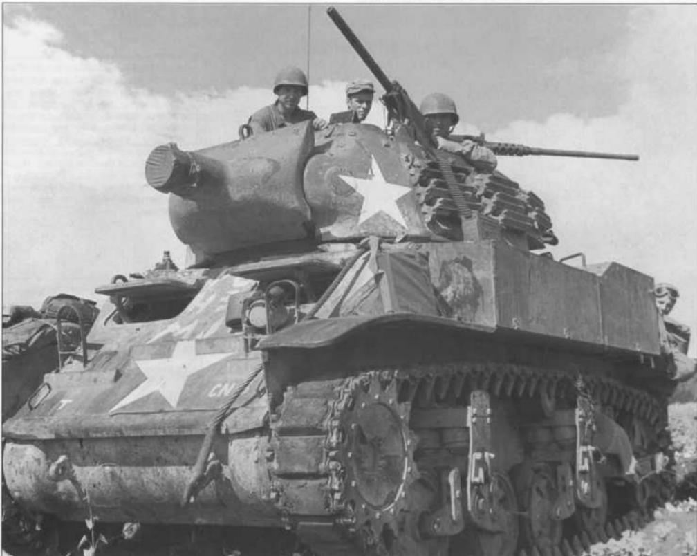
An Army M8 75mm howitzer motor carriage during operations on Saipan. This was based on the M5 light tank chassis, but with a new open-top turret. There were six of these assigned to each armored cavalry squadron, providing fire support to other vehicles in the unit with their short-barreled 75mm howitzer.
