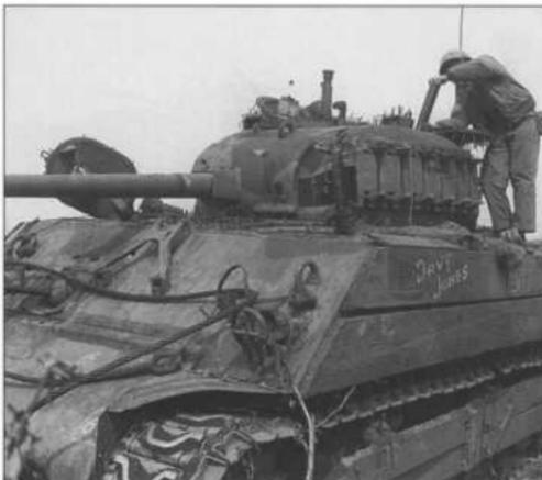
Another view of "Davy Jones" and its crew, providing a better view of the suspension. This tank has "duck-bill" end connectors on the track to provide better floatation in the soft soil. Notice also the planking over the suspension bogies, intended to prevent attacks by Japanese anti-tank teams with satchel charges and other improvised anti-tank weapons.
