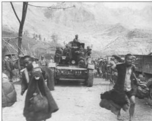
A Chinese T-26 Model 1933 moves along the road at the time of the Japanese offensive in November 1944 near Chin Chen-chaing China. This vehicle shows the location of the standard tactical markings on the tank bow. Notice also that this vehicle is fully equipped with searchlights over the gun barrel.
