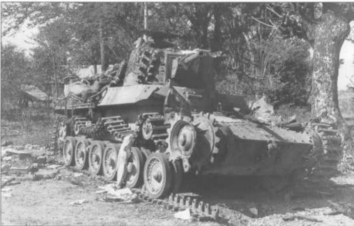
A Japanese column of eight tanks and 30 trucks from the Japanese 2nd Armored Division attempted to push through US lines near Umungan on Luzon on 30 January 1945. This was the lead tank, and it was hit by two bazooka rockets and heavy machine gun fire. One bazooka round shattered the front drive sprocket. One of the curious details here is the use of spare track links by the crew as a form of improvised armor; this was very uncommon on Japanese tanks during the Pacific war.
