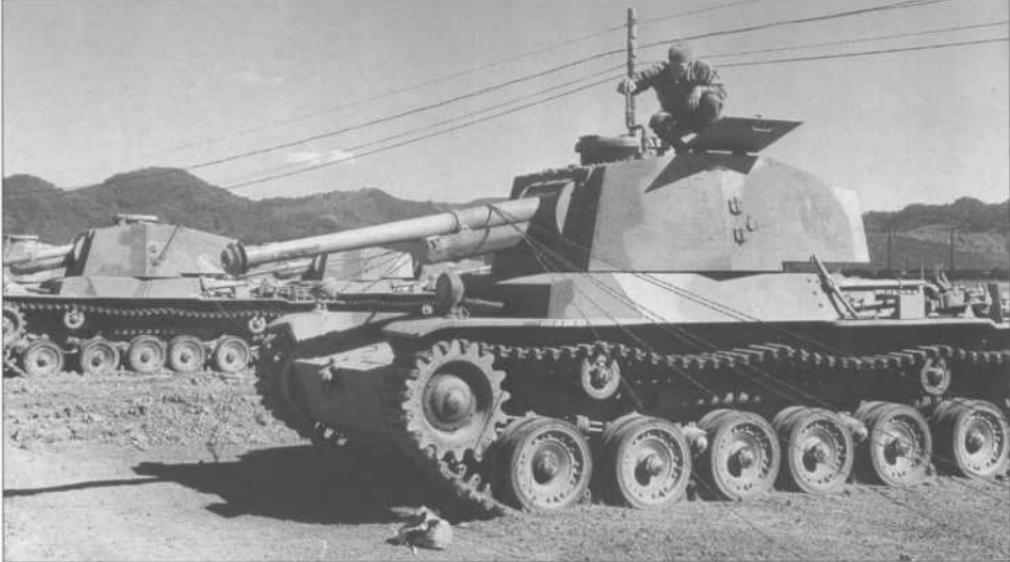
Although the Japanese tanks encountered through most of the Pacific fighting were inferior to the M4 Sherman medium tank, by the end of the war, the Japanese had developed a new and powerful medium tank, the Type 3 Chi-nu armed with a 75mm gun. These were saved for the final defense of the Japanese Home Islands, but ultimately never fired their guns in anger.
