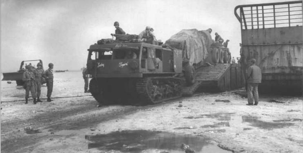
The largest amphibious operation in 1945 was the assault on Okinawa. This is a M4 16-ton high speed tractor towing a 155mm "Long Tom" gun off a landing pier at Keise Shima on 31 March 1945, the day before the main landing. The artillery was deployed on Keise Shima to conduct artillery bombardment prior to the main landing.
