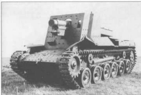
An equally rare vehicle was the Type 4 Ho-ro self-propelled 150mm howitzer which mounted a 150mm howitzer on a Type 97 tank chassis. This was a new assault gun which only entered production in 1944. There were two assigned to the 2nd Armored Division, and they were knocked out in fighting in March 1945. This one was shipped back to the United States for technical evaluation, but it was destroyed during a Korean War scrap drive.
