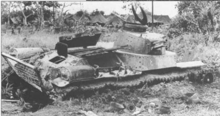
A Type 97 Chi-ha of the 4th Company, 9th Tank Regiment that became bogged down in soft soil during the 16 June attack. Notice that a frame has been attached at the rear of the tank. This was added on many tanks to permit them to carry infantry along during the attack.
