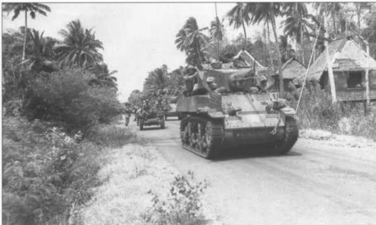
A M5A1 light tank of Co. D, 706th Tank Battalion, leads a motorized column from the 40th Infantry Division shortly after the landings on Negros Island in the Philippines on 29 March 1945. This is a late production model of the M5A1, evident from the cover over the turret side machine gun mounting.
