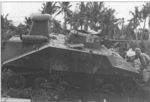
During the Luzon fighting, the Japanese SNLF Marines attempted a major raid behind US lines at Ormoc Bay on 6 January 1945. The attack included Type 2 Ka-mi amphibious tanks of the Kule 101st SNLF, including the one seen here. The stack behind the turret is a deep wading trunk like those used on American tanks to prevent water from flooding the engine. This tank has already shed the two pontoon sections carried on the front and rear which made this tank amphibious.
