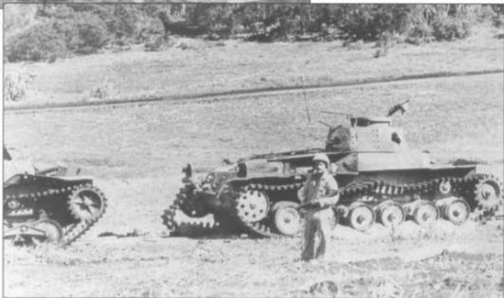
About six Type 97 Chi-ha survived the night attack of the 9th Tank Regiment. This tank of the 5th Company was later knocked out, probably by M5A1 light tanks of the 762nd Tank Battalion. The 57mm gun on this vehicle is missing, and two 37mm hits can be seen immediately below and to the left of the gun mantlet. This view shows the markings of this company: two Japanese flags on the lower bow, and the intricate *kikusui* emblem on the turret side.
