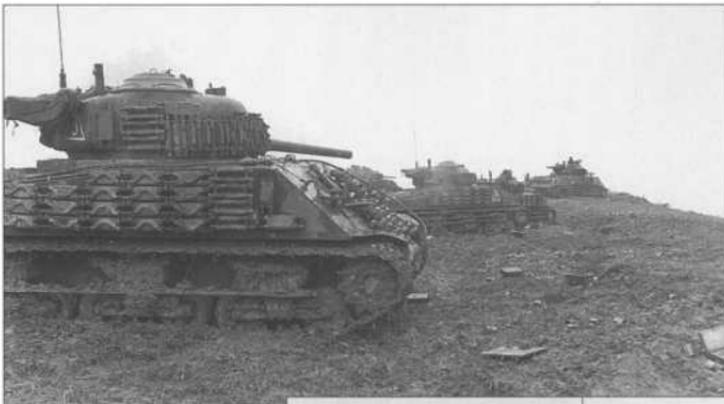
A platoon of M4A2 (W) medium tanks of the Marine 1st Tank Battalion during the fighting near Naha in May 1945. The extensive use of track blocks was intended to protect against anti-tank guns and various types of hand-emplaced anti-tank mines. The suspensions of the tanks were often covered with timber or wood planking to prevent Japanese infantry from striking the thin hull armor with lunge mines or with explosive devices.
