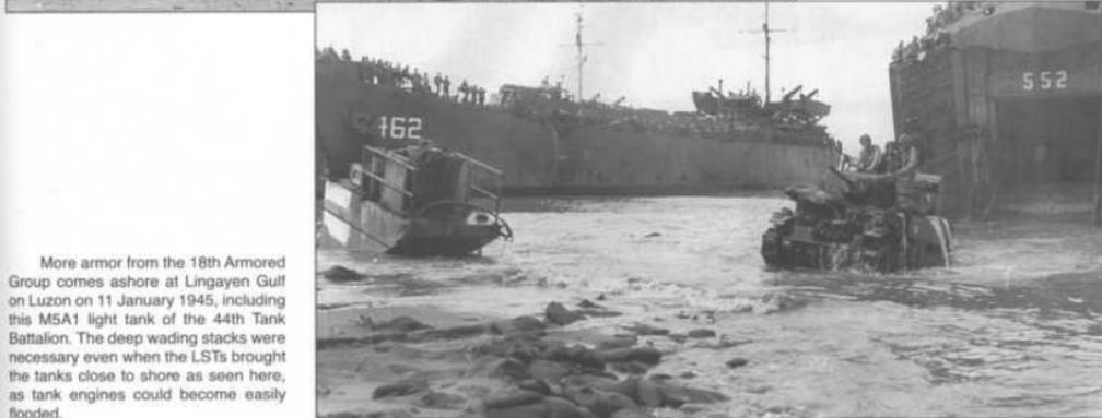
More armor from the 18th Armored Group comes ashore at Lingayen Gulf on Luzon on 11 January 1945, including this M4A1 light tank of the 44th Tank Battalion. The deep wading stacks were necessary even when the LSTs brought the tanks close to shore as seen here, as tank engines could become easily flooded.
