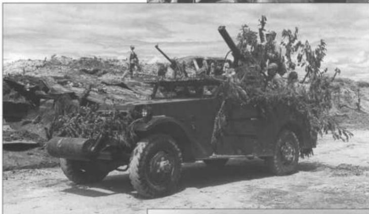
The Chinese Army used a variety of other Lend-Lease equipment, including this camouflaged M3A1 scout car, armed with a water-cooled .50 cal Browning heavy machine gun on an anti-aircraft mount.
