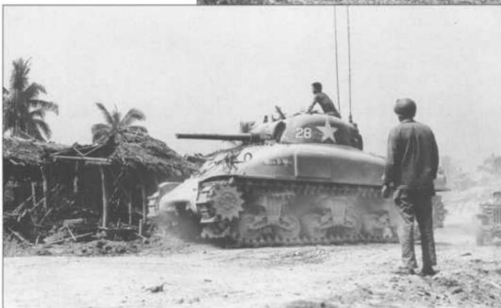
A M4A1 medium tank named "Man O'War" moves through the town of Jualita on 24 October 1944. Notice that the tank has grousers fitted to the track, in an attempt to aid the traction of the smooth rubber block tracks in the frequently encountered mud of Leyte.
