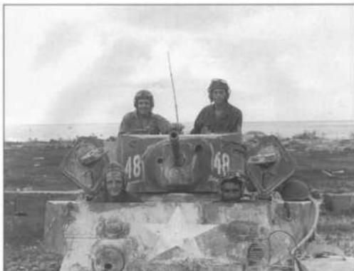
The Army's 762nd Tank Battalion was credited with the most tank kills during the fighting along the Saipan beaches against the Japanese 9th Tank Regiment. This is a M5A1 light tank of Co. D, 762nd Tank Battalion, with the beaches evident behind. Although obsolete by European standards, the M5A1 light tank was more than adequate when faced by any of the lightly armored Japanese tanks.
