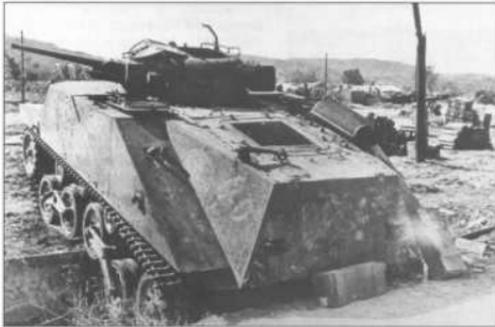
During the night of 15-16 June, the Japanese SNLF marines made their own naval landing near the American invasion beaches on Saipan, attempting to disrupt the US defenses. They were accompanied by a few Type 2 Ka-mi amphibious light tanks. The Type 2 Ka-mi had detachable pontoons at front and rear, and this photo of one of the tanks knocked out in the fighting shows the tank after the pontoons had been dropped.
