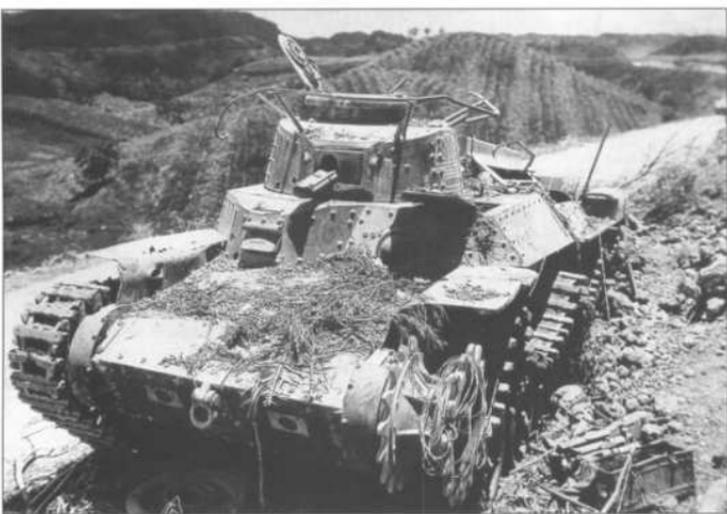
The Saipan campaign was the first encounter where the new Type 97-kai Shinhoto Chi-ha was encountered in significant numbers. Although first deployed in early 1942, the low priority assigned to Japanese tank production meant that few were available in the Central Pacific until 1944. The tank's new 47mm made it capable of defeating the M4 Sherman under the right circumstances. This is a tank of the regimental command platoon, evident from the white band markings around the turret.
