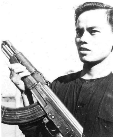
*The AK-47 was the standard hand-held firearm on the Communist side. The Russian-designed gas-operated automatic rifle fired a 7.62mm round. It had an effective range of 400 metres and delivered 30 rounds per magazine. Ruggedly built, it was believed by many*
