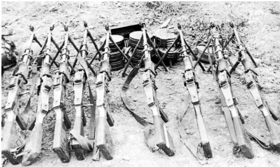
*The Soviet RPD machine gun fired the same ammunition as the American M-60. However, at 10.5 pounds it was less than half as heavy as its counterpart. It was cap-*
