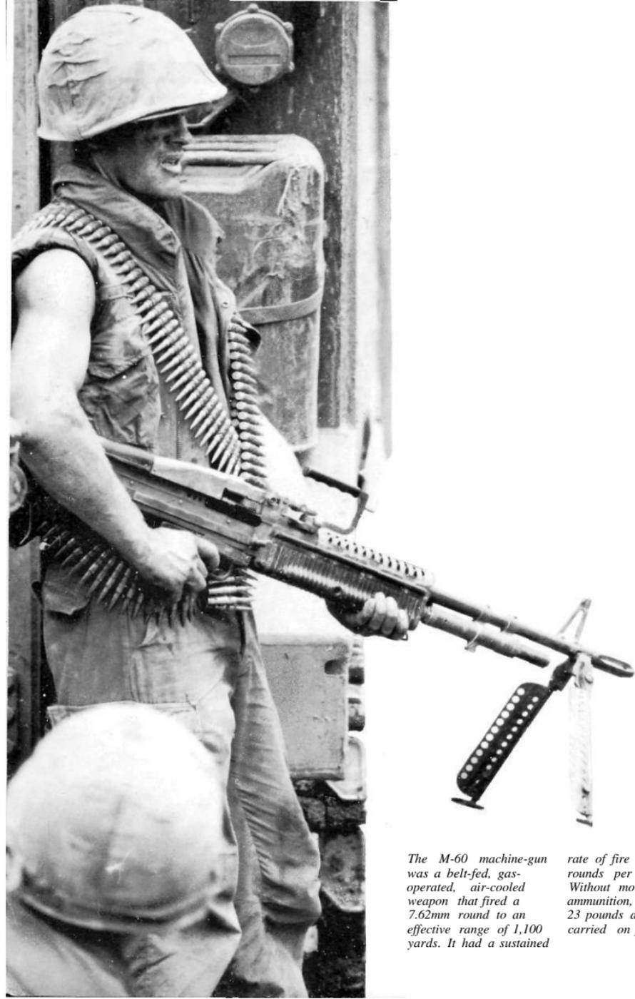
*The M-60 machine-gun was a belt-fed, gas-operated, air-cooled weapon that fired a 7.62mm round to an effective range of 1,100 yards. It had a sustained*
