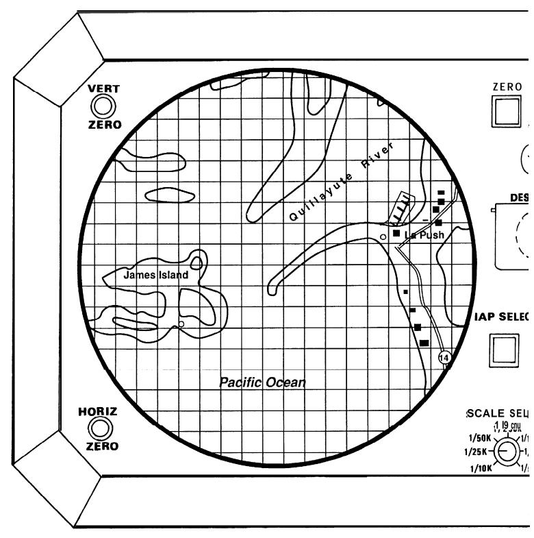
VERT ZERO; Allows adjustment of the displayed map to the unit in the vertical plan.
