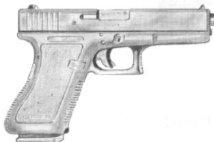
The Glock 20 functions the same as the model 17 above, but is a slightly larger weapon built for the more powerful 10mm round. The model 21 is identical to the 20, but is chambered for the .45in ACP cartridge. Neither has a "plus two" magazine available, but even without them both have the largest magazines available in their calibers.
