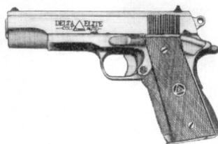
The Delta Elite is a single-action 10mm autoloader based closely on the design of the M1911, below. Combining a tried and true design with a successful new round, it has essentially the same frame and features as its predecessor, including a grip safety and left side manual safety and slide lock. It adds rubber combat grips. Because of its similarity to the M1911 in design and feel, firers used to the older weapon will be comfortable shooting the Delta Elite.
