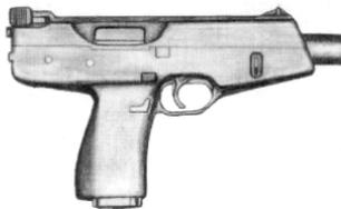
Introduced in 1989, the Steyr SPP (Special Purpose Pistol) is a pistol variant of the TMP, covered under submachineguns later in this text. It is a recoil-operated double-action weapon with synthetic receiver and frame.
