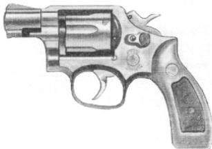
The Model 10 is the most common revolver in the United States, and probably in the world. It is a simple design, with a double-action operation and a swing-out cylinder. It is a very common police weapon in the United States.
