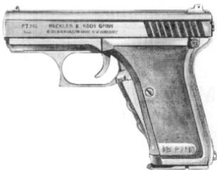
The Heckler & Koch P7 series was created specifically with police use in mind. The design concept called for a weapon that was as safe as possible when carried, but which could be brought to action with a minimum of obstructions. The result is a pistol with a number of unique features.
