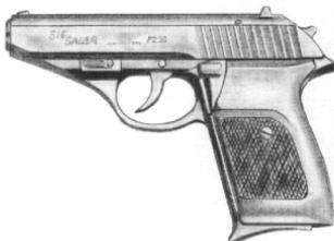
The P230 is a departure from the family of weapons described above. A double-action blowback-operated weapon firing a lighter round, the P230 was designed specifically for police work. It has no external safety lever, but, like other SIG designs, has a non-ambidextrous decocking lever. The P230 is available chambered for .380in Auto or .32in ACP round, and both calibers are available in black or a slightly heavier stainless steel.
