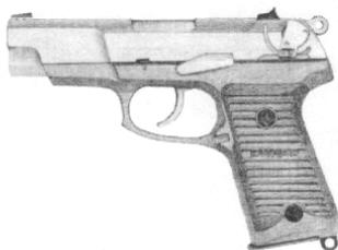
The 9mm P-85 Mark II was introduced in 1987, and is the first Ruger autoloader designed specifically for military applications. It is a double-action, recoil-operated weapon, with an ambidextrous safety and magazine catch. The trigger guard is recurved for a two-handed grip, and is large enough to allow use while wearing gloves. The weapon is normally finished in black, but is available with a stainless steel finish. There is also a variant that replaces the manual safety with a decocking lever.
