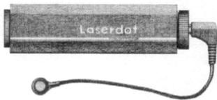
This is a visible-light laser sight designed specifically to withstand the hard conditions and heavy recoils that often go along with military use. It can be fitted beneath the barrel or on top of most longarms, as well as on pistols. It is activated by a pressure switch that connects to the main unit via a 14cm cable, which can be mounted anywhere on the weapon. A toggle switch is also available.
