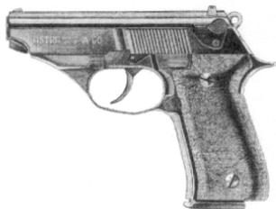
The Astra A-60 is a small, lightweight pistol chambered for either the .380in Auto or .32in ACP round. It has a simple double-action mechanism and operates by blowback. There are safety levers on either side, and the decocking lever can be moved from one side to the other when the weapon is stripped, so it presents no penalty to left-handed firers.
