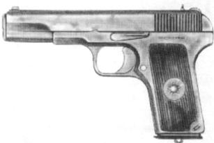
The TT-33 was initially introduced in 1930, but significant changes to the design were made in 1933, giving the weapon its name. The TT-33 is a basic recoil-operated single-action design. It offered no innovations at its introduction, but instead focussed on simplicity of manufacture. The pistol has no safety, but the hammer can be moved to a half-cocked position, locking the slide and trigger. Although obsolete, the TT-33 is still manufactured and used in many ex-Soviet client states.
