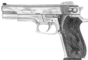
The 5900-series weapons are the largest of the three new series firing the 9mm round. They are functionally identical to the 1000-series weapons above, although they have the added feature of a recurved trigger-guard for improved two-handed grip. The 5903 has an alloy frame and stainless-steel slide, while the 5904 has an alloy frame and carbon steel slide, and is blued. Both slide and frame of the 5906 are made of stainless-steel.
