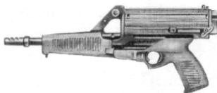
The Calico 950 is a unique pistol in almost every regard. The weapon operates with a two-part, roller-locking bolt similar to that of the CETME and Heckler & Koch rifles (see the introduction to the Assault Rifles section for an explanation of the mechanical operation). The magazine is cylindrical, and sits above the weapon. The pistol is made of lightweight, modern materials, including cast aluminum and glass-fibre reinforced polymers.
