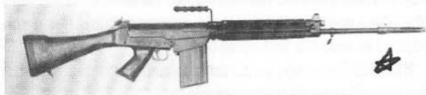
FN FAL with folding carrying handle raised
