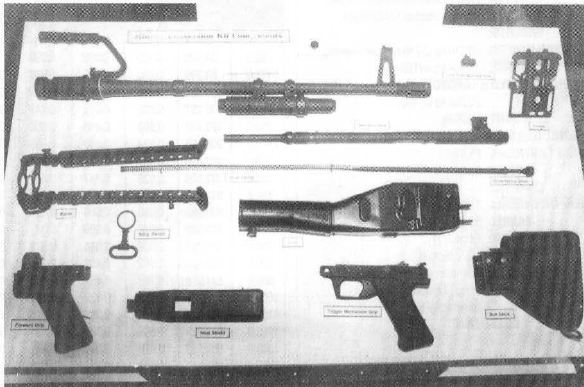
Conversion kit to change the M60 machinegun to the M60E3 configuration
