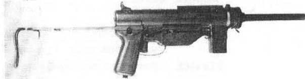
M3A1 with stock extended, no magazine, and the dust cover/safety in the closed/safe position
