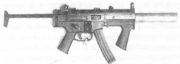
MP-2000 with stock extended and suppressor attached, bolt is locked to the rear on an empty magazine, selector switch on 0, gas selector on high (H)
