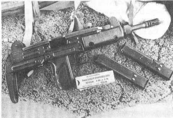
UZI with M16 flash suppressor on the muzzle
