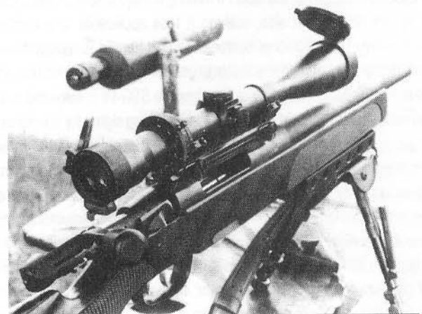
Steyr SSG PII showing the ART IV telescopic sight and its controls
