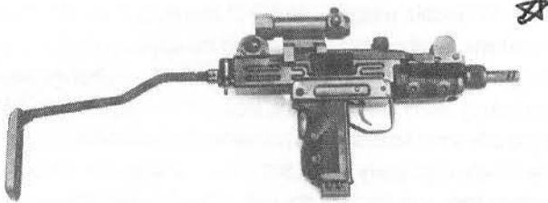
Mini UZI fitted with the Armson OEG sight, with 20 rd magazine
