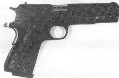
M1911A1: Note the base pad extending from bottom of magazine
