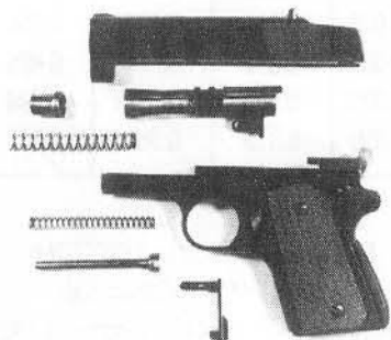
A field stripped Detonics Combat Master
