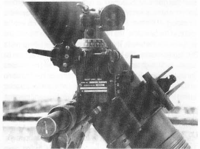
L16 Mortar, closeup of sight mounting on left side of bipod showing the M64 sight
