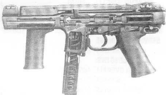
Spectre M-4, left side cutaway view
