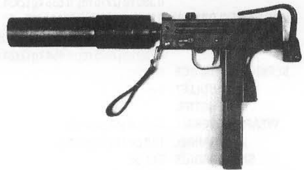
Ingram M11 with MAC suppressor mounted and 32 rd magazine, selector set to full automatic and bolt in forward position
