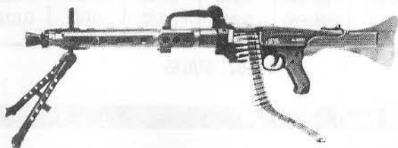
CETME Ameli with ammunition belt inserted and bipod extended
