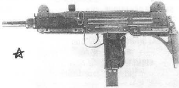
UZI with Hebrew markings, fitted with a 25 rd magazine and metal stock (folded)
