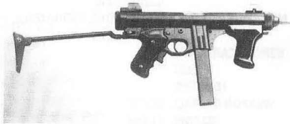
PM-12S with stock extended and bolt forward
