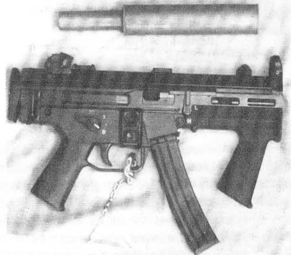
MP-2000 with suppressor unmounted, selector set to 0 (safe) and gas selector set to high pressure. Retracting stock is slightly extended
