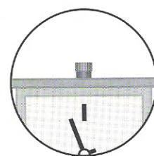
Distress signal activated by pulling out winding knob
