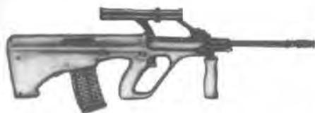
An unusual and exotic-looking weapon, the AUG (Armee Universal Gewehr) is a bullpup assault rifle firing the 5.56mm round. It is ergonomically designed, and has modular components allowing it to be converted to a light machinegun, a submachinegun, and a shorter carbine version, by simply changing barrels and breech mechanisms. All of the AUG weapons are covered in this text (see pages 76 and 134).
