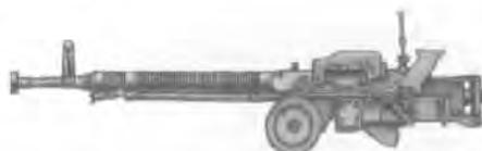
Introduced in 1969, the NSV is a heavy machinegun that has slowly been replacing the DShKM, above. It is a gas-operated weapon firing the same round as its predecessor. It is essentially the same in features and use, but is substantially lighter and features a quick-change barrel.
