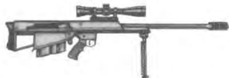
The M90 is a smaller, lighter version of the M82, and is bolt-action. Because there is no semiautomatic mechanism to absorb recoil, the M90 is fitted with a muzzle brake that would look at home on a tank. It has no iron sights, but is equipped with a mount that will take almost any scope.
