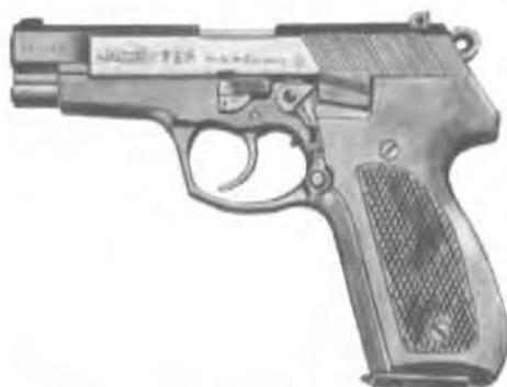
The P-88 was introduced in 1988, and is another double-action, recoil-operated 9mm autoloader. Its simple controls are fully ambidextrous, with a combined decocker/slide release lever mounted on the receiver and the magazine catch on the grip. The safety is internal, and no manual safety is fitted. The trigger guard is checkered to give a good two-handed grip, but not recurved. It has been evaluated by several military organizations, including the British army.
