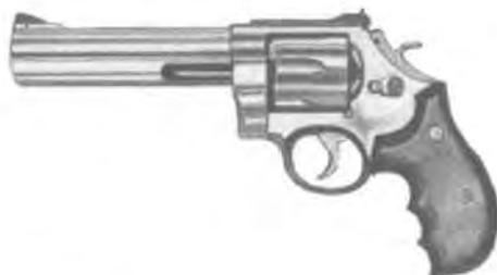
The Model 29 is a large revolver firing the .44in Magnum round, and is without a doubt one of the most powerful handguns around. It is a double-action weapon with a swing-out cylinder. The power of the round requires a very sturdy weapon, and the Model 29 can be difficult to control, due to the sheer size and weight of the pistol as well as the noise and impact of firing. When properly controlled, however, it is quite accurate.
