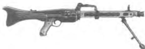
Introduced in 1982, the Ameli is a blowback-operated light machinegun based on the roller-locked bolt design of the CETME and HK rifles. It features an integral bipod, an easily-changed barrel, and a rate of fire that can be adjusted between two settings by making a minor internal change. It is compact and easy to strip and assemble. A lightweight version that makes maximum use of alloy components is available. The Ameli is in service with the Spanish and Mexican armies.
