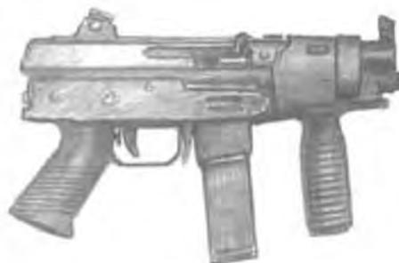
Designed for covert and bodyguard operations, the Mini-S.A.F. is an extra-short version of the S.A.F. 9mm, below. It features a shortened barrel and a vertical forward handgrip. The shoulder stock featured on the S.A.F. 9mm is also missing, replaced by a shoulder strap for carrying the weapon and providing tension to steady it when firing. The standard magazine is 20 rounds, but the weapon can use the S.A.F. 9mm's 30-round magazine. In all other ways, it functions identically to the S.A.F. 9mm.
