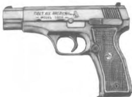
Unlike most other Cold autoloaders, the Colt 2000 is a new design not based directly on the M1911 (page 31). A double-action, recoil-operated pistol, it features an ambidextrous magazine catch and an internal safety that negates the need for a manual safety. Although the slide is made of steel, the receiver is polymer, keeping weight down.
