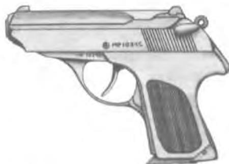
The PSM is a Soviet knock-off of the Walther PP, and is issued to the police, internal security, and military police forces throughout the ex-Soviet bloc. It was introduced in the early 1980s, and is a double-action blowback weapon with a narrow design for concealability. The PSM fires the 5.45mm round, which has a bottle-necked shell (common in rifle rounds, but unusual in pistol ammunition).
