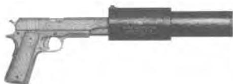
Built from a heavily-modified Colt M1911A1, the Colt .45 Silenced has an integral suppressor that is attached to the slide rather than the barrel. (Despite the name, this weapon is actually suppressed, not silenced.) This gives the slide enough weight for the weapon to operate on blowback instead of recoil, and the result is an extremely reliable, accurate weapon that operates very quietly while firing standard .45in ACP cartridges.
