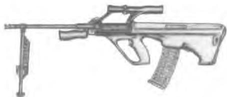
This weapon is the light machinegun version of the Steyr AUG system, and is functionally the same as the AUG assault rifle (page 98) and other members of the family. It is fitted with a heavier, longer barrel than the assault rifle, and fires from the open rather than closed bolt position. It can also be obtained without the AUG's optical sight, having a mounting bar for some other sighting mechanism in its place—this is referred to as the HBAR/T version.
