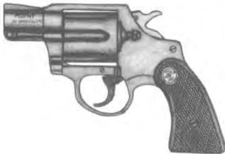
First produced in the 1960s, the Colt Agent is one of the smallest revolvers firing the .38in Special round. It is a double-action pistol with small, rounded features for easy draw and concealability. It can be a little uncomfortable to shoot, especially for large-handed firers, but it is reliable and rugged.
