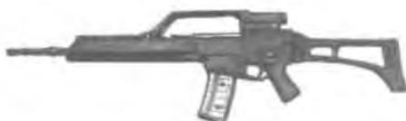
Adopted by the German army in 1996, shortly after the G11 program was abandoned, the G36 is a gas-operated rifle of relatively conventional design, despite its radical appearance. What is unusual about it, at least for an HK weapon, is that it functions by a rotating bolt system similar to that of the M16A2 and hundreds of other autoloading rifles—the roller-locking breech design common to almost all HK longarms was discarded to reduce weight.
