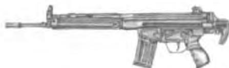
The G33E is a 5.56mm assault rifle based closely upon the G3. In fact, many of its parts, including the trigger mechanism and bolt, are interchangeable with the latter. Normally made with single-shot and full automatic fire options, the G33E can be modified to allow a three round burst. It is available with a fixed or collapsible stock. The G33K is a shortened version, with a collapsible stock and cut-down barrel.
