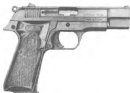
The PA15 is a 9mm autoloader in service with the French army. It operates by blowback, with an unusual delay device that causes the barrel to rotate as the slide goes back. The safety, slide lock, and magazine catch are all mounted on the left side, making the weapon inconvenient for left-handed users. MAB went out of business in the mid-1980s, so the PA15 is no longer produced.
