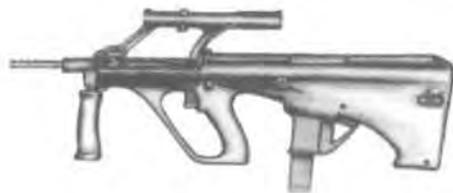
This is a 9mm weapon based on the AUG assault rifle. In fact, many of the components are the same, and the submachinegun can be ordered as a conversion kit for an existing rifle. The weapon is blowback-operated, and fires from a closed bolt. This, along with its long barrel, make the AUG Para an exceptionally accurate submachinegun.
