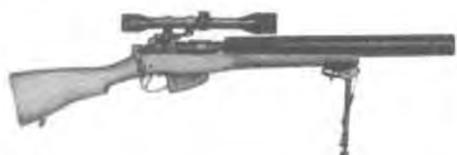
The LEI DeLisle is based on a silent weapon used during the Second World War. It fires the .45in ACP round, ideally suited for silent firing due to its very low velocity. A bolt-action weapon, the Mark 3 is exceptionally quiet, producing only the noise of a firing pin striking the primer. An unusual feature of the Mark 3 is its magazine, which collects the spent shell casings in a compartment behind the live rounds.
