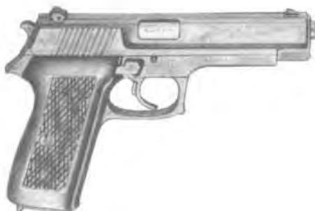
This pistol was specifically designed with military and police applications in mind. It is a recoil-operated double-action weapon of rugged design, with a recurved grip and trigger-guard for two-handed use and a reputation for low recoil, good balance, and accuracy.
