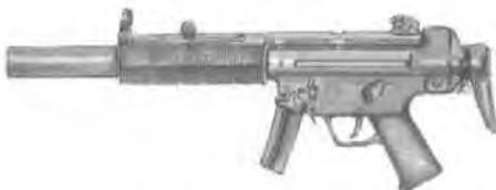
The MP5SD series weapons are versions of the MP5 with integral silencers. They operate in the exact same manner as the MP5. A number of small holes in the barrel bleed away cartridge gases, reducing the velocity of the bullet to below the speed of sound by the time it leaves the barrel. This allows the weapon to fire standard ammunition, while making the MP5 the quietest off-the-shelf silenced submachinegun made.
