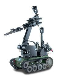
Bomb Disposal Robot, Size: Trashcan, Movement: Treads,
