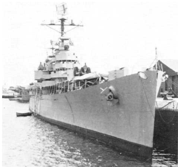
Some of the considerable modifications made to the cruiser General Belgrano can be seen here: note two quadruple Sea Cat SAM launchers on bridge wings, Dutch LW08 surveillance radar forward and DA radar aft. The Sea Cat launchers were controlled by two Italian RTN10 FC systems. When HMS Conqueror's two World War II-vintage Mk 8 torpedos hit her on the port side, one amidships and one near the bows, the bow collapsed and folded down almost to the 6in. gun turret; the second torpedo appeared to have broken her back. (Dr. R. Scheina via MARS)
