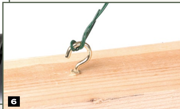
Step 6.) Wrap the other loose ends around the secured eyehook (a nail works as well).
